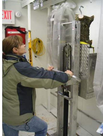
Figure 5. Using a hydraulic lift to suspend a log from the ceiling rack. Photo Dave Holden
